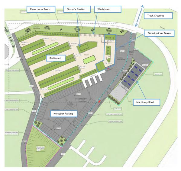
Figure 4 – Proposed Temporary Stableyard Site Plan (Dwg 0509 Extract)
