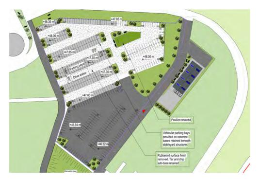
Figure 7 – Parking area on Temporary Stableyard site (Dwg 0507 Extract)
