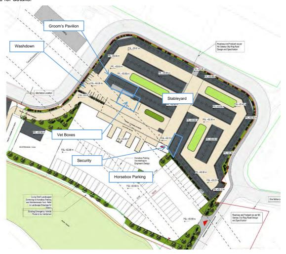
Figure 9 – Proposed Permanent Stableyard Site Layout (Dwg 0516 Extract)
